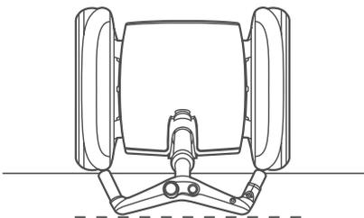
4. Loosen the Height Adjustment Collar and extend the Handlebar/Control Shaft Assembly approximately 6 inches (15 cm). Then, tighten the Height Adjustment Collar.
