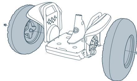
require multiple attempts as the wheel hub is seated tightly into the Gearbox taper.)
