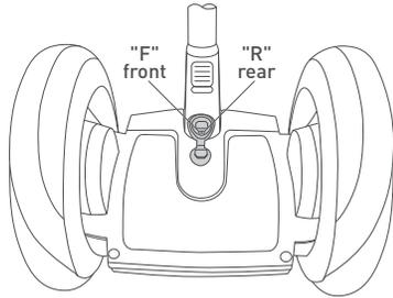
The Control Shaft Base has two LED (Light Emitting Diode) charging indicators located below the Charge Port.
