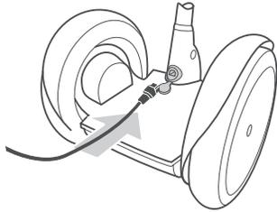
In order to maintain the best performance from your Segway HT Battery Packs, fully charge your Battery Packs for at least twelve hours, once a month, or once every twelve hours of operation— whichever comes first. Make sure that your Battery Packs are within the specified charging temperature range when charging.
