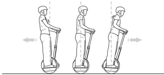
The Segway HT works like the human body. If you lean forward, you take a step forward to keep your balance. If you lean back, you step back. Substitute wheels for feet, and you have an empowered pedestrian on a Segway HT.
