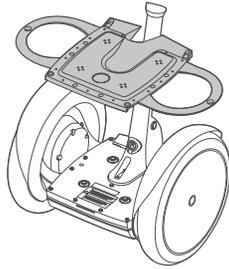
1. Make sure the Segway HT is powered off and not plugged in. It is unsafe to perform this procedure while the Segway HT is powered on or charging.
